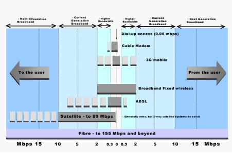
Figure 13: Bandwidth supplied by delivery technologies
